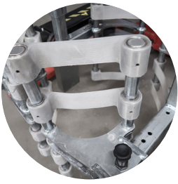
Specially developed polyurethane gripping pads
